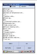
Click in the box to select parameters in which you want to view the datastream, the selected items will be marked with '√'. You could select "CHAR" or "GRAPH" to view datastream in different form as you want, as shown on the left.
