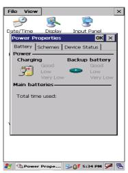
Note: Click the start menu " \* "at the bottom left of the interface to find "control panel". With a new window pops up, double click "Power", and the power properties interface appears. You can also double click the icon for 'battery' in the taskbar to open the Power Properties interface, as shown above.
