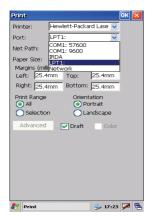
In this screen, select "Hewlett-Packard Laser Jet" in the drop-down menu of Printer. Then select "LPT1:" in the drop-down menu of Port, as shown on the left.
