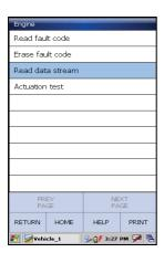
Click [Read data stream] on the function menu to read the datastream from ECU, as shown on the left.
